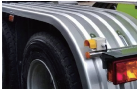
Mudguard Aluminum Dual-Rear-Wheel Mudguard 2nd Steering Axle Mudguard Complete Subframe Covering
