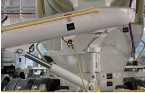
Hydraulic Chute Ram with Built-in Safety Valve (control by remote) Effortless operation.
